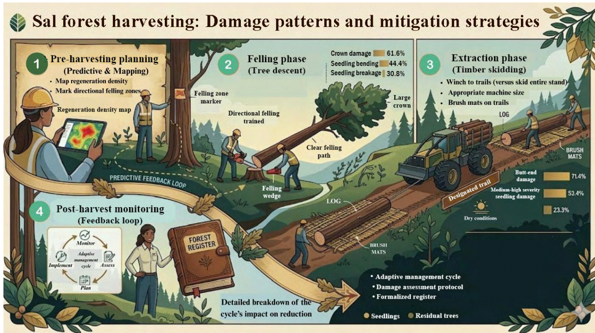
Fig. 6 Conceptual framework linking observed damage patterns to targeted mitigation strategies during felling and timber extraction in Sal-dominated forests. The figure illustrates the operational phases (left column), primary damage types documented in this study (center, with percentages), and evidence-based interventions (right column) to minimize residual plant damage.
