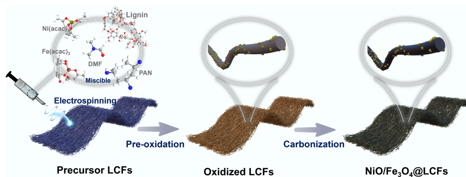
Fig. 1 Schematic diagram of the synthesis of NiO/Fe 3 O 4 @LCFs.
