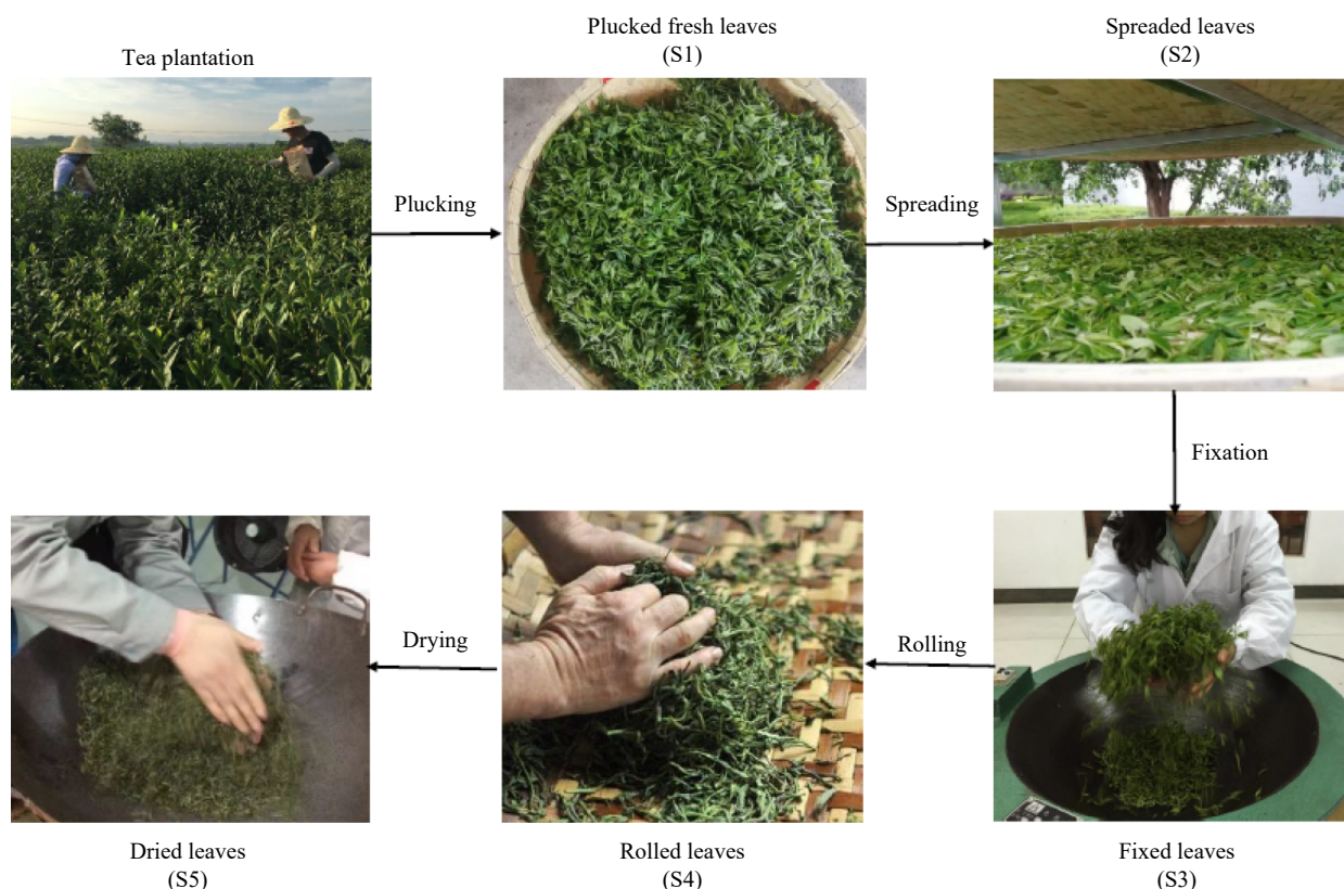
Fig. 1 The Yuhua tea (stir-fried green tea) processing of 'Yinshuang' tea leaves. Photographs show the five major stages of the Yuhua tea manufacturing process: plucking (S1), spreading (S2), fixation (S3), rolling (S4) and drying (S5).
