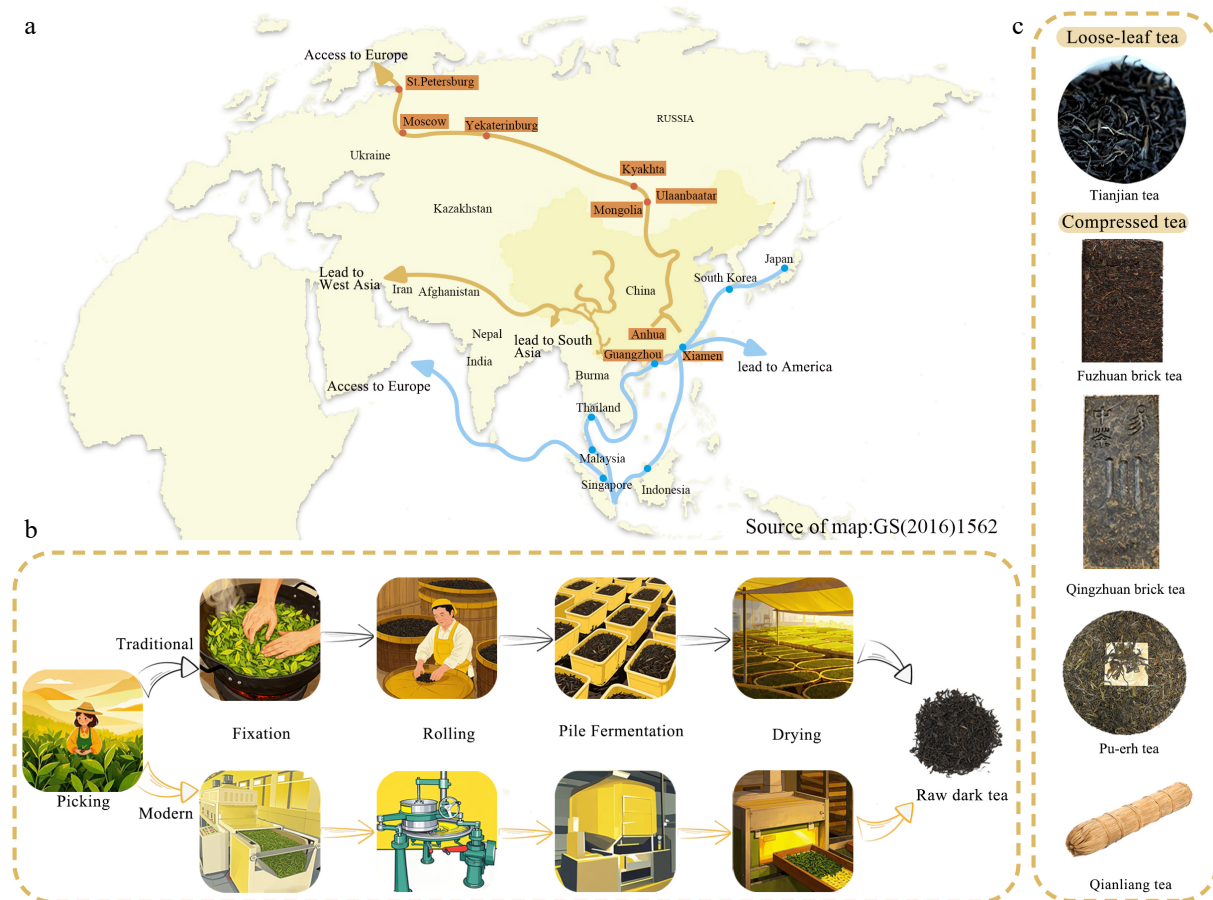
Fig. 1 The overview of historical routes, manufacturing, and morphological types of dark tea. (a) Dark tea trade routes: overland (orange) transported to Asia and Europe; maritime (blue) transported to Southeast Asia, Europe, and the Americas. (b) Traditional and modern processes of dark tea production. (c) Morphological types of dark tea: loose-leaf and compressed.
