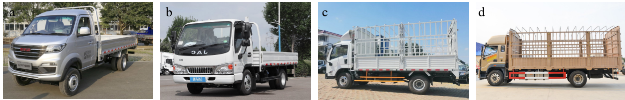
Fig. 1 Examples of different types of two-axle trucks. (a) Micro truck. (b) Light truck. (c) Medium truck. (d) Heavy truck.
