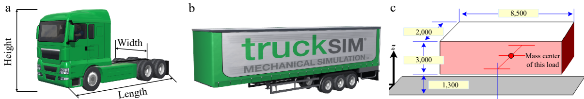
Fig. 2 Simulate vehicle models. (a) Tractor model. (b) Semi-trailer model. (c) Load model.
