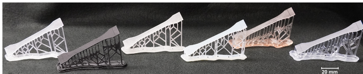
FIGURE 6 | 3D-printed type 1BA specimens, along with a supporting structure to ensure a well-defined macroscopic orientation during printing, made from various resins (from left to right: Clear V4, Black V4, High Temp V2, Durable V2, Surgical Guide V1, and BioMed Clear V1). Scale bar: 20 mm.
