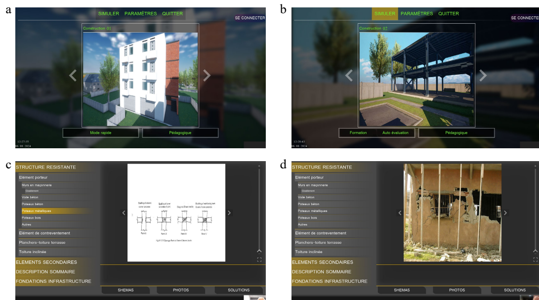
Fig. 7 DIMA virtual training and qualification centre with the purpose of learning, testing/validating, and qualifying. (a) Virtual training center: typology masonry. (b) Virtual training center: typology metal. (c) Pathology: damage of nodes. (d) Pathology: damage of walls.
