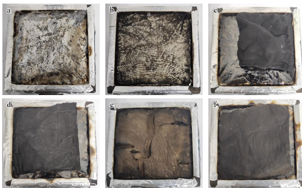
Fig. 14 CCT photos of raw and treated cotton fabrics. (a) COT, (b) \text{SiO}_2 @COT, (c) AMP@COT, (d) AMP- \text{SiO}_2 @COT, (e) \text{SiO}_2 -KH570@COT, (f) AMP- \text{SiO}_2 -KH570@COT.
