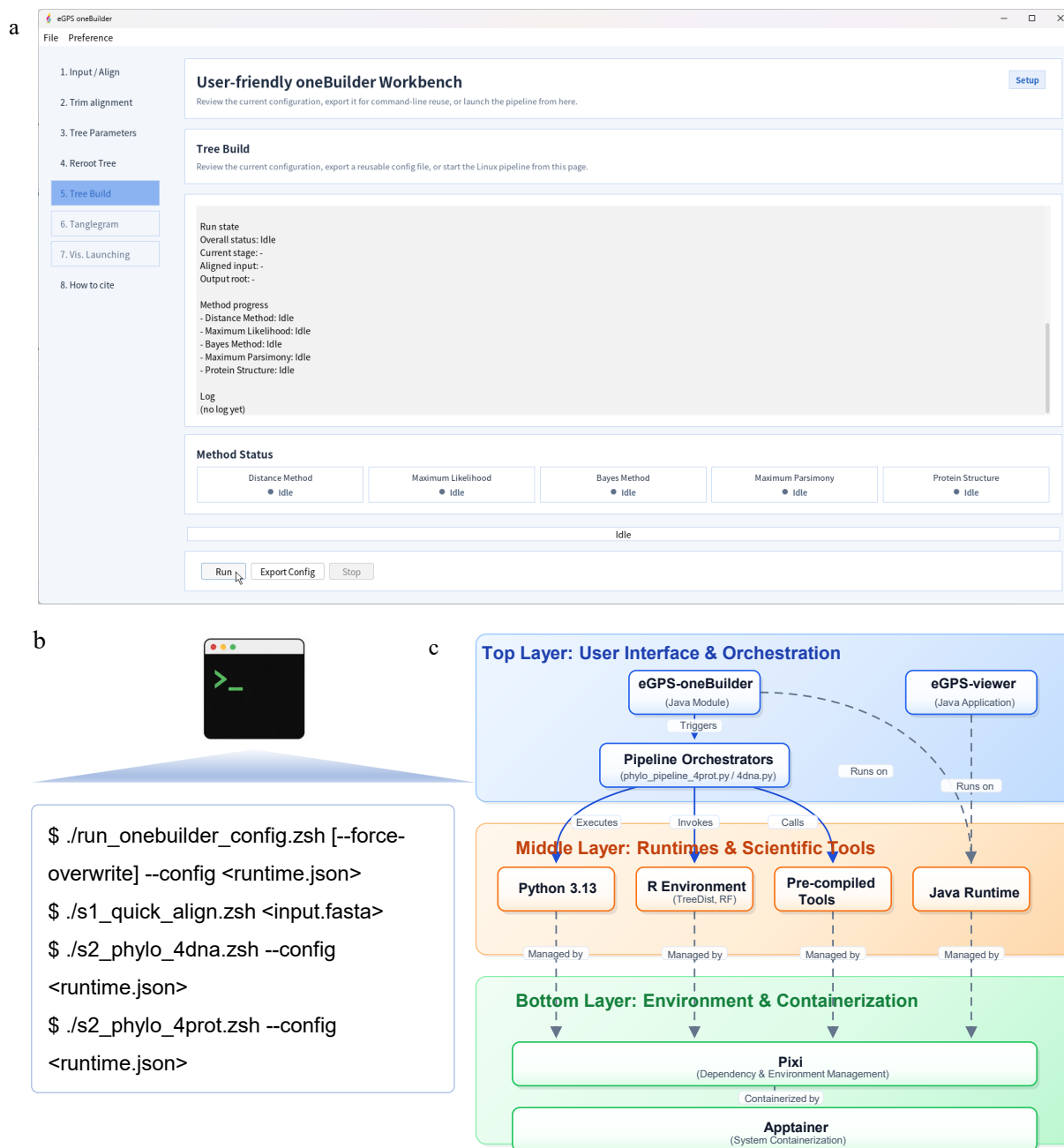
Fig. 1 Overview of the user-friendly oriented design of a reproducible one-stop GUI-CLI bridge workflow. (a) eGPS-oneBuilder GUI organizes input/alignment, parameter configuration, tree building, and downstream visualization in a guided tabbed workflow. The steps are organized as liner workflows, and the tab 'Tree Build' demonstrates the core step of the tree-building method with broad methodological paradigms: distance-based, parsimony, likelihood-based, and Bayesian approaches. For protein sequences, the protein structure-based clustering tree is also supported. (b) GUI-selected settings are exported as a reusable runtime JSON file and replayed by command-line scripts. The command-line interface is allowed for bioinformaticians. Users can save the configuration from the GUI and replay the analysis without intervention. Thus, the eGPS-oneBuilder implements a reproducible one-stop GUI-CLI bridge. Please see the 'Application to human WNT and FZD paralogs' section for a practical application scenario. (c) The software solves the installation pinpoint by invoking the apptainer ( https://apptainer.org ) and pixi ( https://pixi.prefix.dev/latest ) technology. The architecture of the software is structured into three layers: a top layer for user interfaces and workflow orchestration (eGPS-oneBuilder runs one), a middle layer providing essential runtimes (Java, Python, R) and analytical tools, and a bottom layer ensuring reproducible environments via Pixi and Apptainer. The dashed line means direct runs on or program dependencies, while the round rectangles represent the entities of packages. eGPS-oneBuilder is run on Linux, while the eGPS-viewer is portable and not limited to the results of eGPS-oneBuilder.
