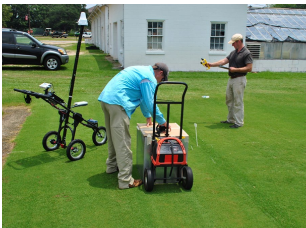
Fig. 2 Examples of ground-based phenotyping devices used in turfgrass breeding and research. Left: pushcart with multispectral sensor; middle: light box with digital camera; right: hand-held NDVI meter. (Photo credit: Brian Schwartz).
