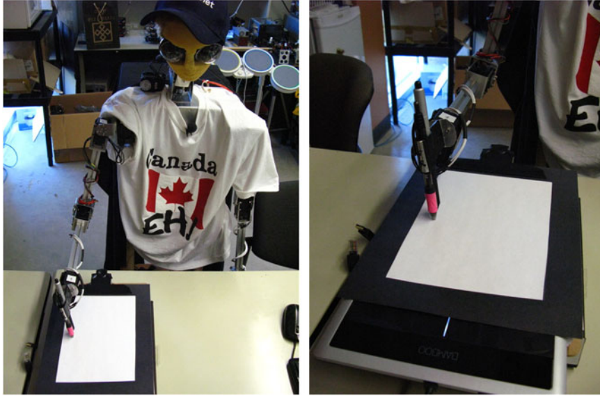
Figure 7. Experimental setup using a Wacom Bamboo tablet (CTH640M), Betty, camera and pen.
