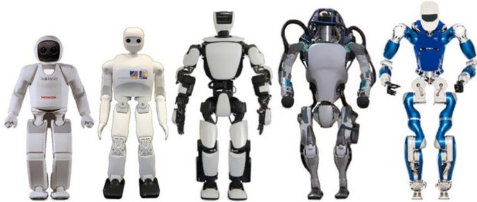
Figure 3 Some well-developed humanoid robots in terms of dynamic bipedal walk and control. From left to right: Honda Asimo, Nimbro-OP2X, Toyota THR3, Boston Dynamics Atlas, DLR-TORO
