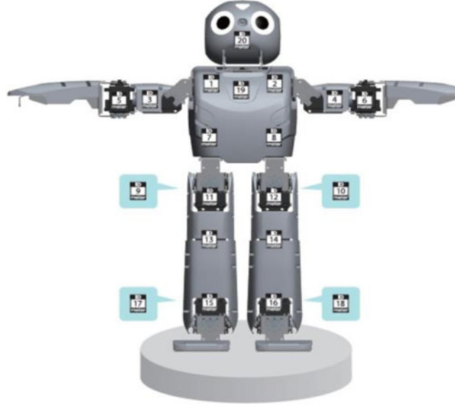
Figure 1 Schematic of the DARwIn-OP servomotor numerically assigned positions
