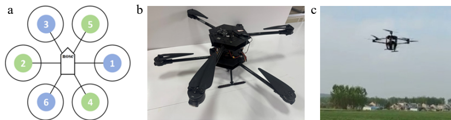
Fig. 14 (a) 'X' layout control scheme; (b) prototype of the novel hexacopter configuration; (c) flight test.
