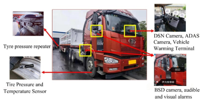
Fig. 4 Hardware system for dynamic risk management data collection of dangerous chemical vehicles.
