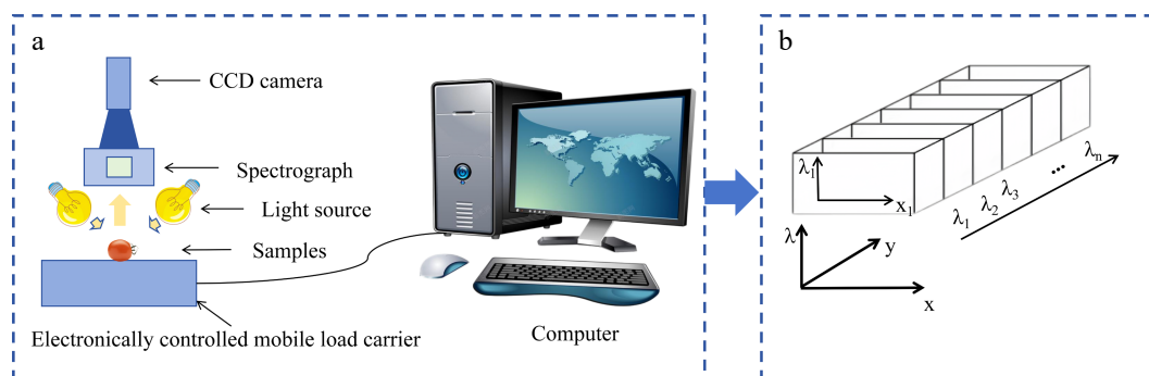
Fig. 2 Schematic diagram of the working principle of a hyperspectral imaging system. (a) Schematic diagram of system optical path and components. (b) Schematic diagram of hyperspectral data cube.
