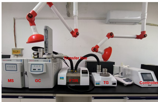
Fig. 1 Photograph of the TG-FTIR-GC/MS experimental setup.
