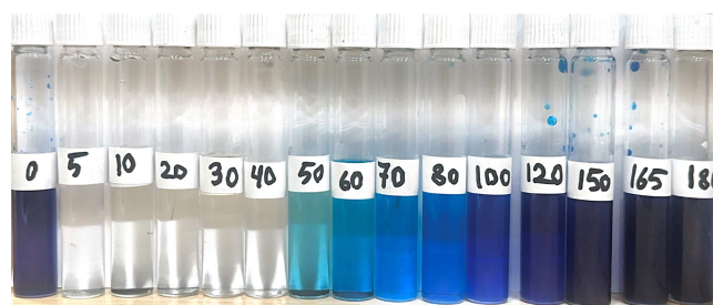
Fig. 17 MB adsorption experiment in a fixed bed column over 180 min.
