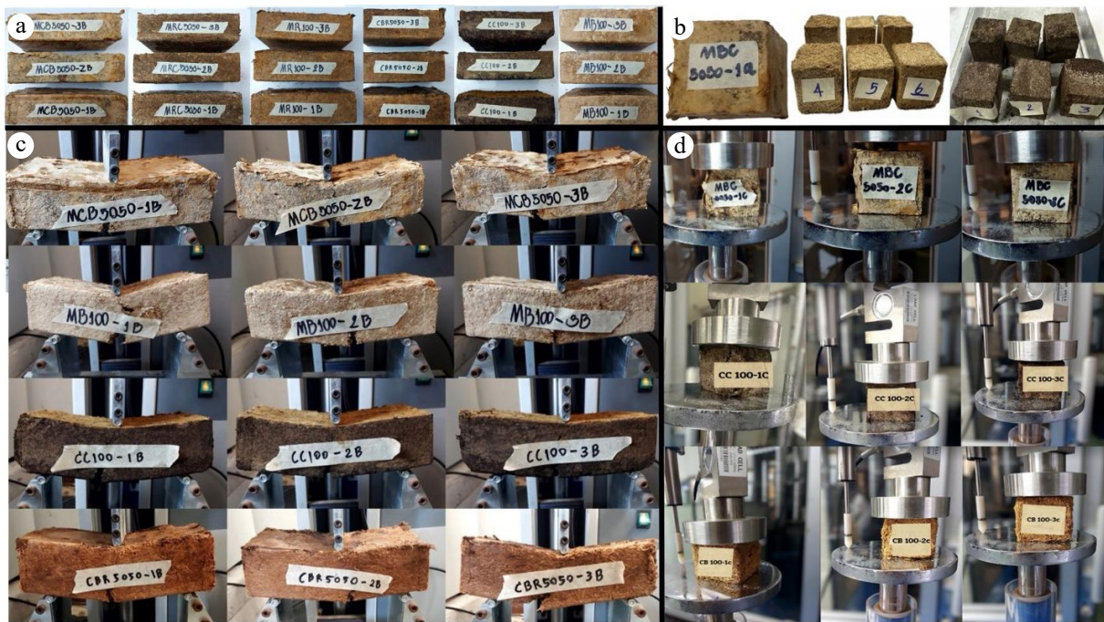
Fig. 3 Visual representation of mycelium-based block samples before testing, during testing, and after failure for modulus of rupture and compressive strength. (a) Test blocks for modulus of rupture prior to testing. (b) Test blocks for compressive strength prior to testing. (c) Samples after failure during modulus of rupture testing. (d) Samples during compressive strength testing.
