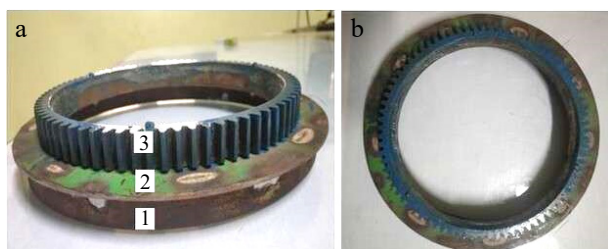
Fig. 1 (a) Front view of upper unit: 1. circular flat; 2. circular plate; 3. ring gear. (b) Top view of the upper unit.
