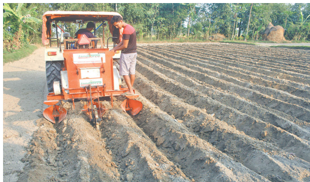
Fig. 4 Potato planter (adapted from Rajbansi [8] ).
