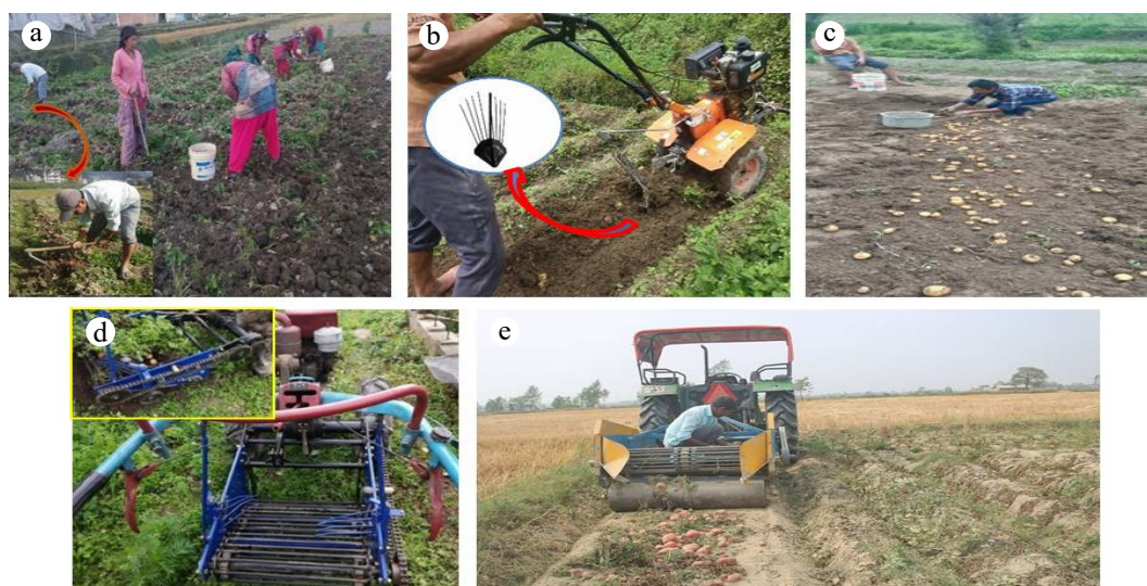
Fig. 5 (a) Manual digging. (b) Mini tiller digger. (c) Collection of digger harvested potatoes. (d) Power tiller digger. (e) Four-wheel tractor attached potato digger (Image 'e' adapted from Bidari [13] ).
