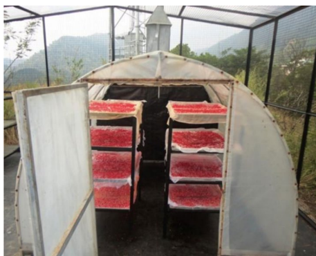
Fig. 4 This image depicts a sample of wild pomegranate arils being dried in a solar tunnel drier. Reprinted from Thakur et al. [102] .
